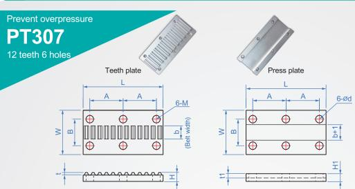
Material Finish AS White anode Aluminum alloy A6061 AB Black anode
